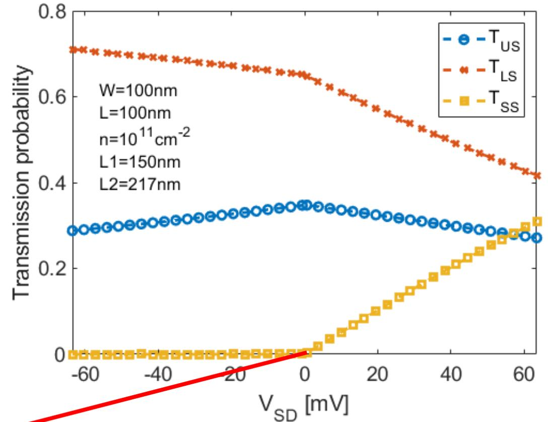
If  $V_{SD} > 0$   $T_{SS}$  can be non null even if  $L_2 > L_1 \left(1 + \left(\frac{W}{L_1}\right)^2\right)$  is satisfied
