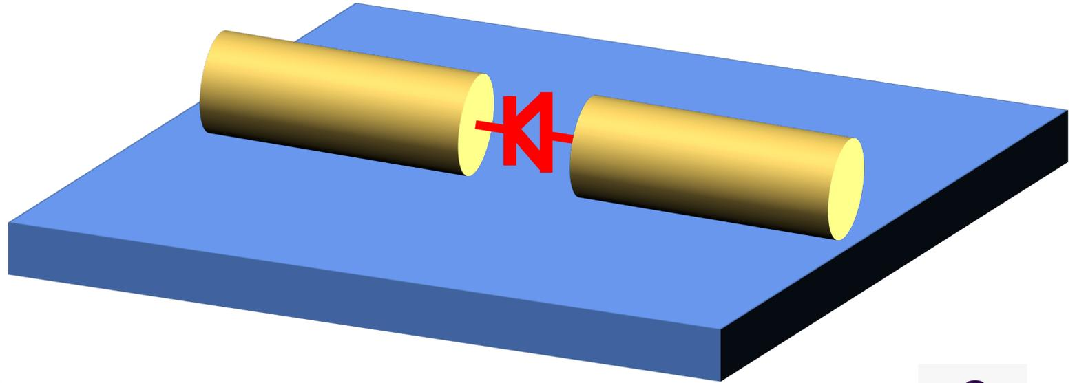
Roughly speaking, when one halves the gap width the field between terminals doubles
