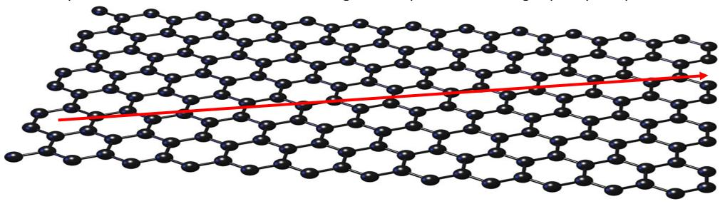
For high-quality graphene samples, particularly those encapsulated in hexagonal boron nitride (h-BN), the mean free path at room temperature can range between **0.5 to 1 micrometer (µm)**
