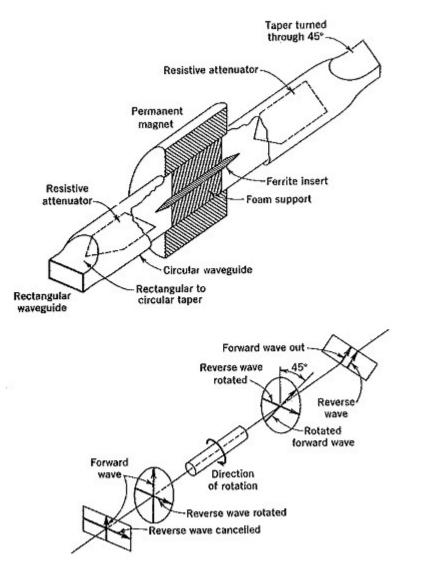
Another example, even "older", is the use of ferrites in microwave waveguides, to obtain non-reciprocal functionalities (isolators, circulators).
