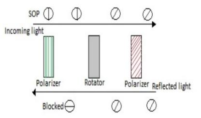
The key for the isolator effect is the nonreciprocal rotation of the forward and backward propagating light – a very uncommon effect in normal optical components!
